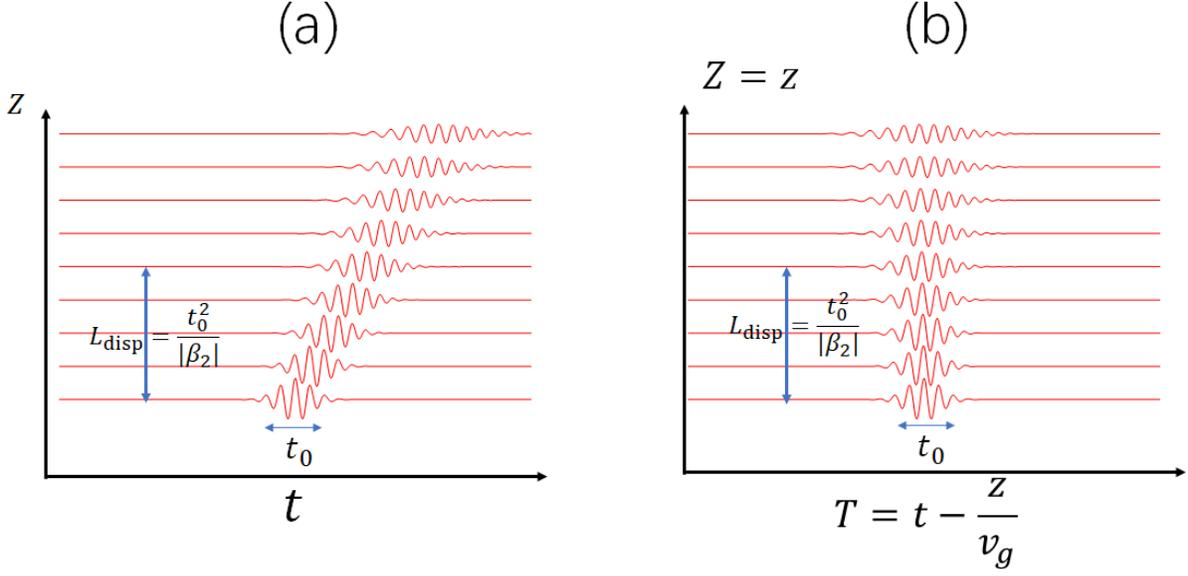
图 11. Dispersion of a Gaussian pulse in (a)  $t - z$  coordinate and (b)  $T - Z$  coordinate. Here  $\beta_2 > 0$ .
