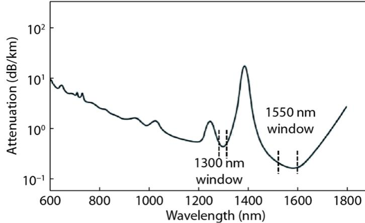
图 13. Telecom windows for fiber-optical communication (from online).
