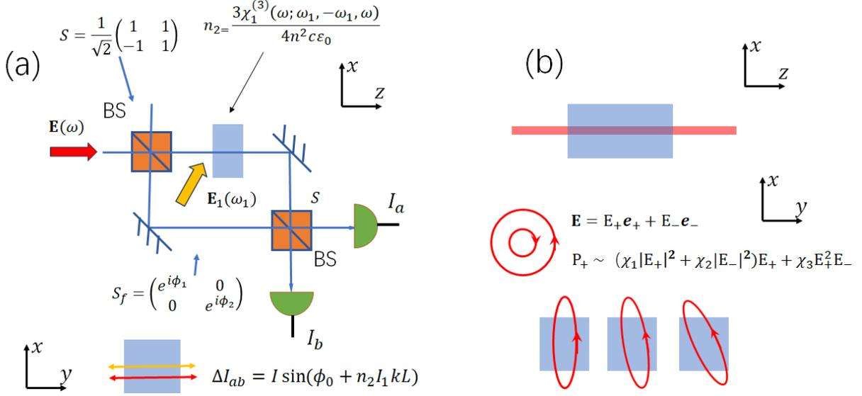
图 1. (a): Mach-Zehnder Interferometer to perform non-demolishing  $I_1$  intensity measurement using Kerr effect. (b): SR: Self-rotation of elliptical light.
