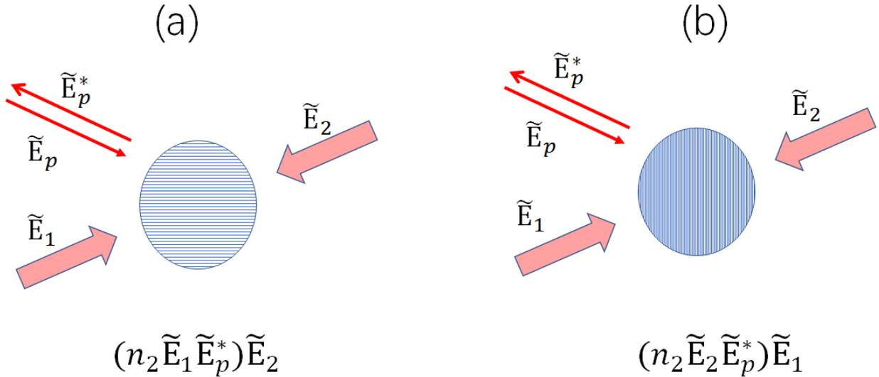
图 4. Optical phase conjugation as dynamic holography. (a) and (b) are two co-existing diffraction processes that convert the incoming  $\tilde{E}_p$  into its time-reversal beam.
