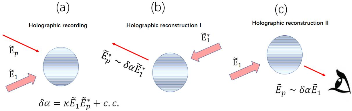
图 5. Principle of optical Holography. (a): recording of hologram. (b): reconstructing the time-reversed output. (c): reconstructing the original field.
