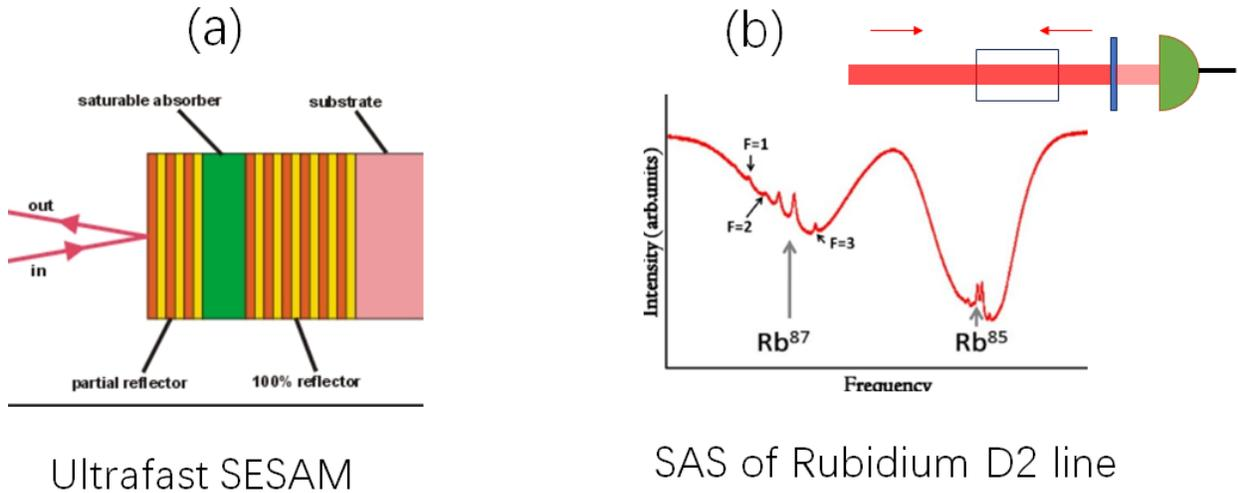
图 8. (a): Semiconductor Saturation Absorption Mirror (From online) (b): Saturation absorption spectroscopy of Rubidium Vapor (Lamb Dips)
