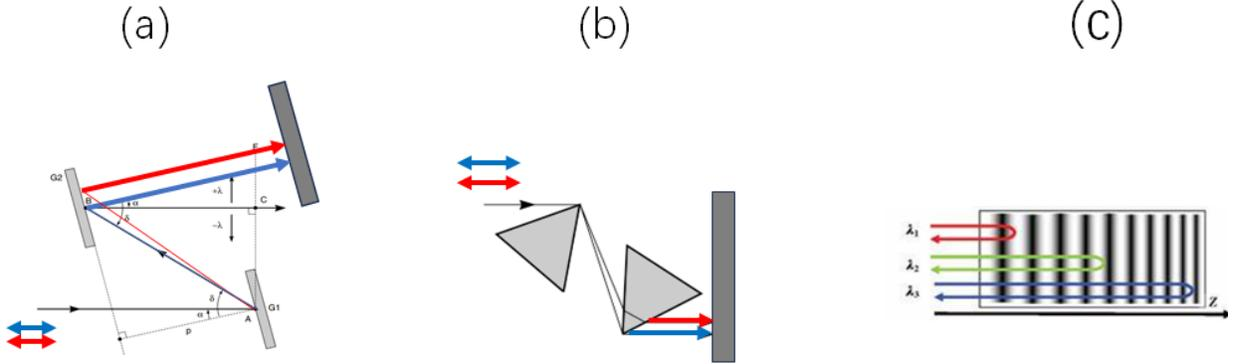
图 14. Dispersion compensation with (a): Grating pair; (b) Prism pair; (c) Chirped Bragg mirror. Here  $\bar{\beta}_{\text{eff}}$  is negative for (a), positive for (c) (both from New Book). But for (b),  $\bar{\beta}_{\text{eff}}$  can be positive or negative, depending on how deep the light rays enter the prisms (from online).
