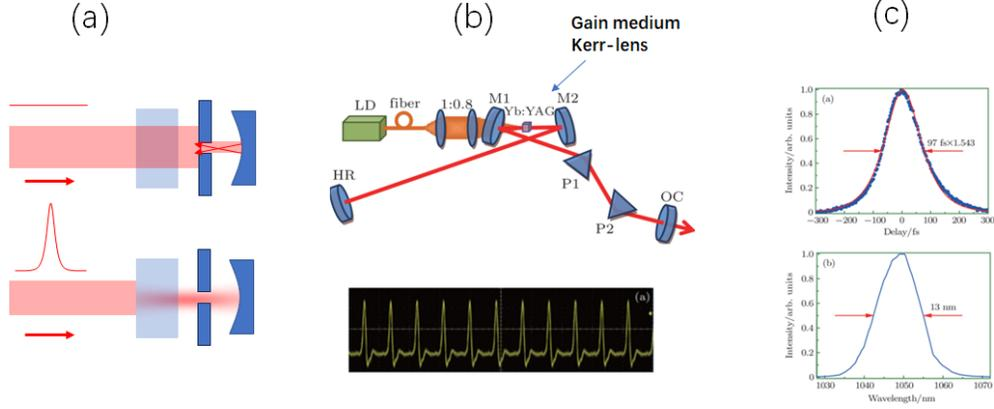
图 16. Kerr-Lens mode-locked laser example. (a): The setup (top) and fast-detector readout of the pulsed output(bottom). (b) Auto-correlation (top) and spectrum (bottom). From Gao et al, Chinese Physics B, 2016, 25(2): 024205.
