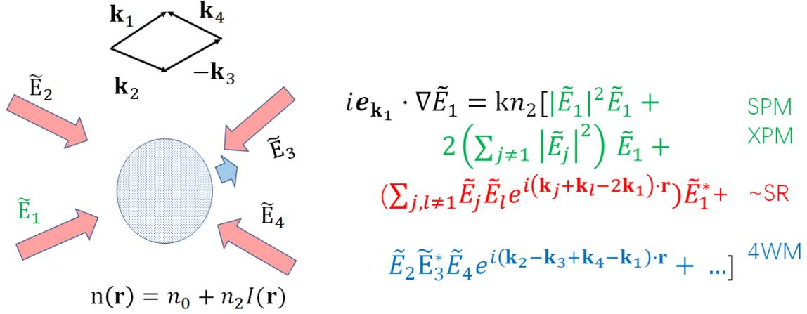
图 3. Grating picture of degenerate 4-wave mixing. The four beams  $\tilde{E}_{1,2,3,4}$  forms interference pattern in space, generating index gratings. Here we are particularly interested in the "4WM"-term marked in blue: The grating formed by  $\tilde{E}_{2,3}$  interference diffracts  $\tilde{E}_4$  to  $\mathbf{k}_1$  direction, if  $\mathbf{k}_1 = \mathbf{k}_2 - \mathbf{k}_3 + \mathbf{k}_4$ .
