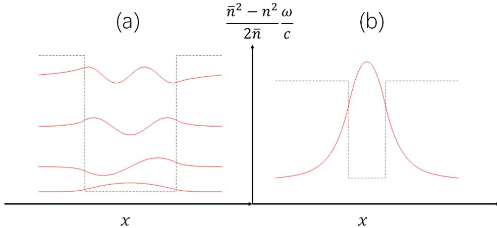
图 9. (a): Transverse mode profiles  $\tilde{E}(x)$  for a multi-mode waveguide. (b): Transverse mode profile  $\tilde{E}(x)$  for a single-mode waveguide.
