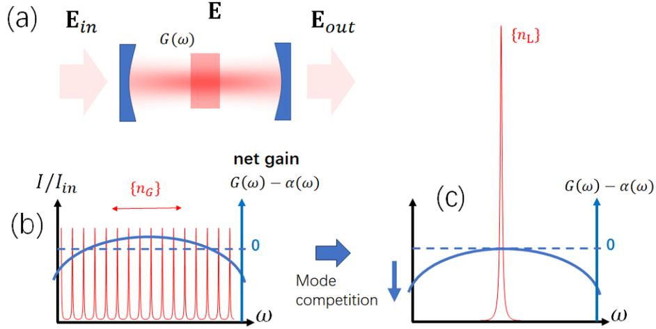
图 15. Generation of single-mode Continuous-Wave Laser.
