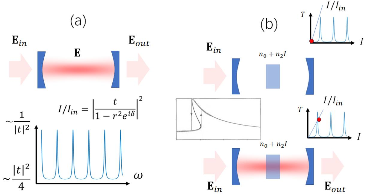
图 7. (a): Transmission spectrum of a Fabry-Perot Cavity. (b): Optical bistability. The inset plot from Powers book showing the bistability curve.
