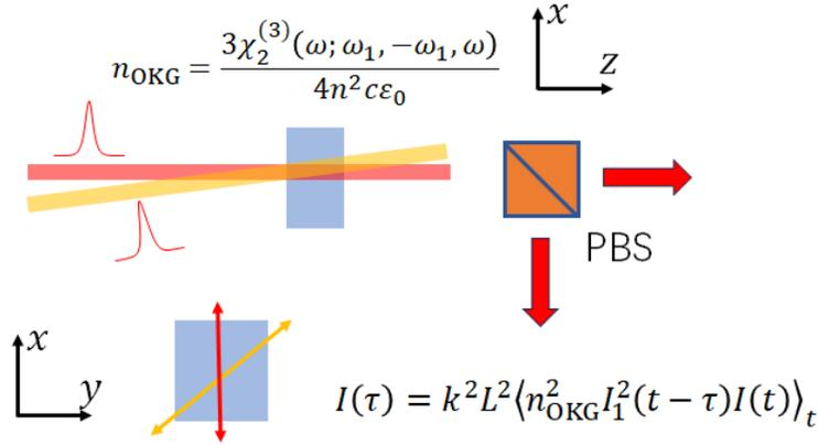
图 2. Ultrafast Optical Kerr gate.
